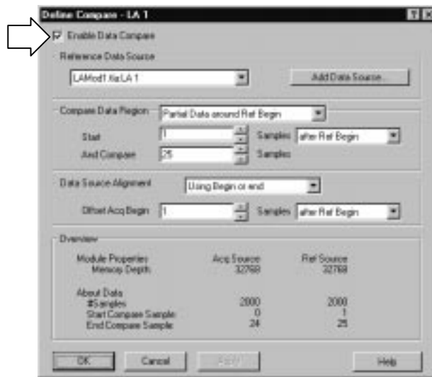
Figure 3–6: Enabling data compare
