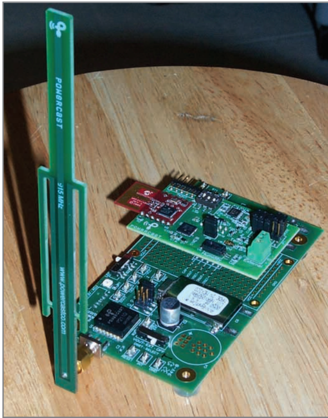
Photo 3 —The Powercast wireless (power and data) sensor comprises the '2110 EVB energy-harvesting baseboard, an antenna (omnidirectional shown here) to capture the transmitted power, and the wireless sensor board comprising an MCU, IEEE 802.15.4 radio, and trio of sensors (temperature, humidity, and light).
