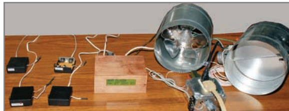
Photo 1 —The complete basement humidity control system is assembled on a table. The heart of the system is the small wooden case in the center, which contains the iMCO evaluation board and associated electronics. The humidity/temperature sensors are on the left. The control box and vent control devices are on the right.
