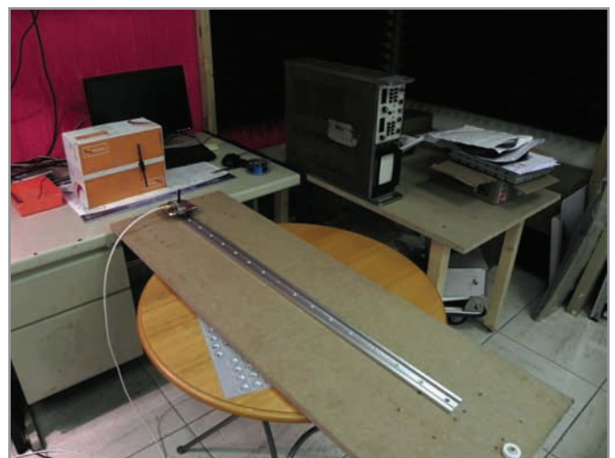
Photo 3 —You can see the reflector I added to get the plot shown in Figure 3b . This is simply a 19" instrument put vertically 50 cm from the antennas. It's a small environmental change, but it has a huge impact.
