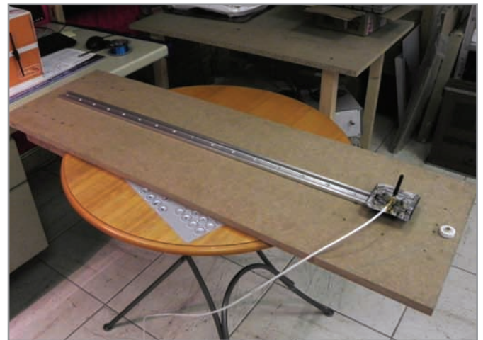
Photo 1 —The rail is 1 m long, which allows for a transmission distance from 20 cm to 1.20 m. You can see that the receiving antenna is fixed on a small ground plane to avoid ground effects. It is gently pulled with a fishing line.
