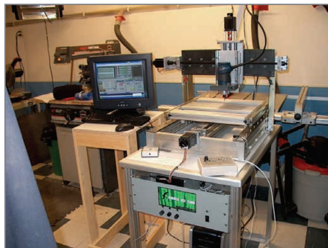
Photo 5 —My moving table CNC router, shown in my home carpentry shop
