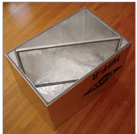
Photo 1 —A simple rectangular box serves as an oven. The box is 36 × 24 × 26-inch on the outside, with 1-inch thick walls made of aluminum-sheathed foam insulating board. The lid sitting inside the box seals against the top edge with two adjoining strips of felt insulation.
