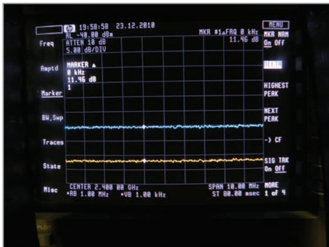
Photo 4 —This is the measurement shown on my trusty HP70210C high-end spectrum analyzer. The yellow signal is the noise level measured when the noise source is switched off. The blue is when it's on. The difference, measured with delta markers, is 11.46 dB which allows us to calculate the noise figure of the amplifier under test.
