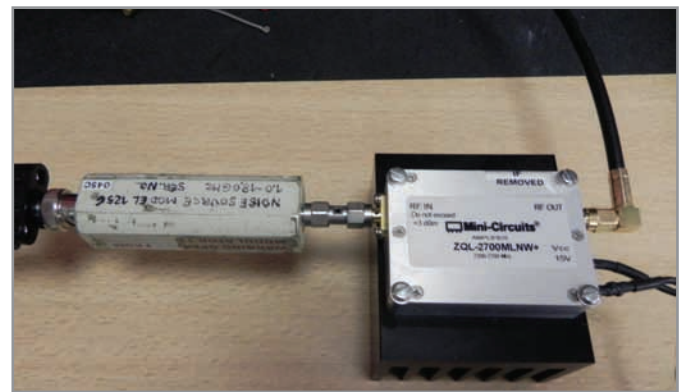
Photo 3 —This is my test setup. The noise source is connected to a Mini-Circuits low-noise, 2.2- to 2.7-GHz amplifier. The output of the amplifier is connected to a spectrum analyzer. Lastly, two DC power supplies are driving the noise source and the amplifier, respectively.
