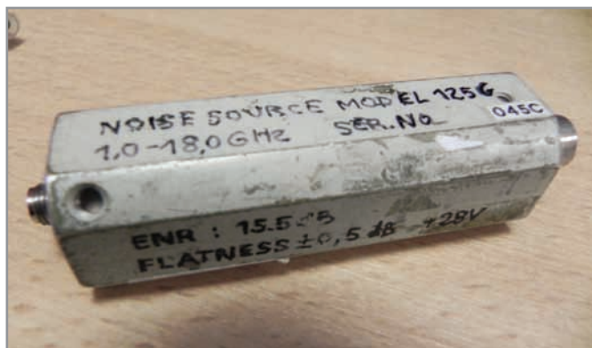
Photo 2 —This old noise source has an unknown supplier. (Maybe Marconi?) It isn’t very pretty, but it works. Fortunately, it was supplied with its ENR value (here 15.5 dB). Such a source has a DC voltage input, usually 28 V, through a BNC connector, and an RF SMA or N output connector.
