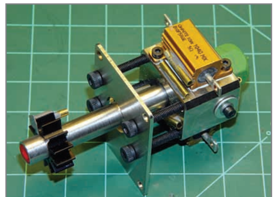
Photo 1 —The MakerBot Plastruder MK5 head uses a pair of aluminum-cased resistors as heating elements. Solid 3-mm plastic filament enters the red PTFE tube, melts as it passes through the Thermal Core block, and extrudes through a 0.5-mm brass nozzle with green PTFE coating. I added the small brass tubes to hold thermocouple beads at key points on the extruder.
