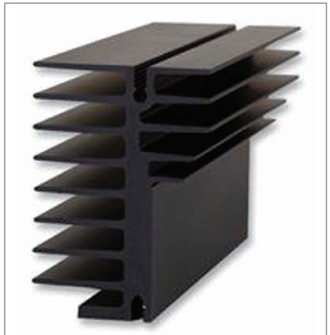
Photo 2 —This 54 × 38 × 100 mm Aavid Thermalloy O5518-100B heatsink gives you what is actually a 2.2°C/W heatsink for natural convection mode.
