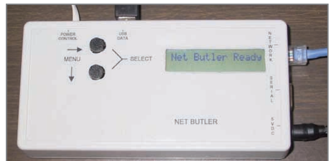
Photo 1 —Take a look at the finished Net Butler design. You can see the various cables leading to the network and the printers.
