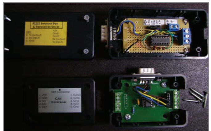
Photo 4 —The CAN and RS-232 custom breakout transceiver boards. Both were designed, built, and debugged. (They were not implemented before the DesignStellaris challenge deadline submission date.)
