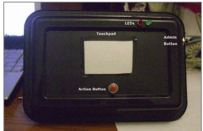
Photo 1 —The password security system prototype consists of a Synaptics touchpad, two push buttons, two LEDs, and a USB connection that provides a simple interface to enter and set passwords.
