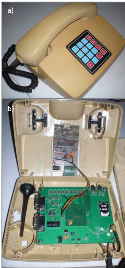
Photo 1 —Don't let the retro casing fool you (a). Inside is a Microchip Technology PIC24FJ64GA002 microcontroller, a GSM board with an antenna, and a connected keypad (b).
