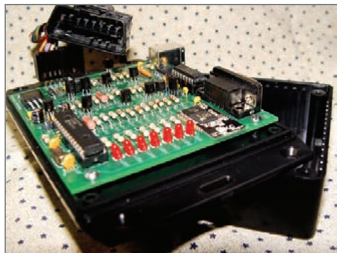
Photo 3 —This project offers experimenters access to their vehicle's private diary via the industry-mandated OBD-II connector.
