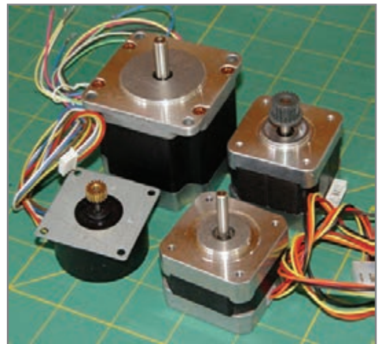
Photo 1 —This assortment of four-, five-, and six-wire stepper motors from my collection represents only a small fraction of the available designs. The largest motor is a NEMA 23 size, the two on the right are NEMA 17, and the smallest one, from my surplus heap, has a custom case.
