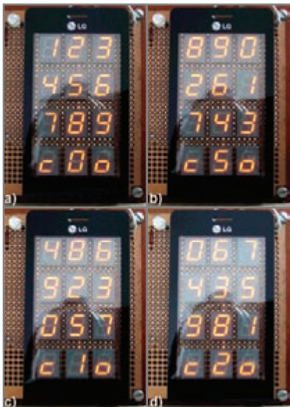
Photo 3 —The standard keypad layout shows up during system start-up (a). Later, only random keypad patterns are displayed (b, c, and d). Because seven-segment displays can't present * or # symbols, these symbols are substituted with "c" (for Clear) and "o" (for OK), respectively.
