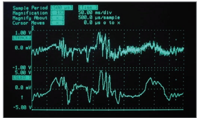
Photo 5 —Here the player is being bumped rather firmly. The tracking system can't keep up and loses synchronization for about 200 ms before it recovers.
