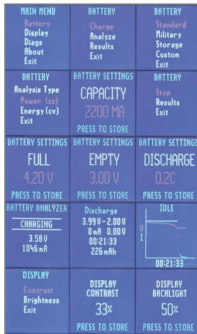
Photo 2—The battery analyzer's menu-driven display
