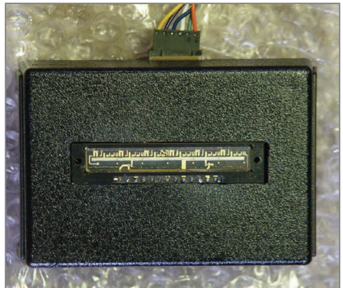
Photo 1 —The TAOS TSL1406R is a 768 x 1 linear sensor array that has a built-in hold function that enables the last pixel samples to be temporarily stored while a new exposure is being taken. The stored analog samples are clocked out during the new exposure. The analog samples are therefore representative of the previous exposure period.
