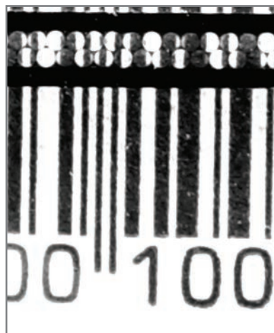
Photo 2 —A close-up of the individual lenses in a strip of SELFOC lens array (SLA) held above the surface of a barcode photo. When affixed properly between the linear array and object to be read, it focuses the image of the object upon the array's linear elements.
