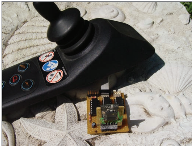
Photo 3 —The joystick normally interfaces to the VR1 with a 0.1" 2 x 4 square pin header. This photo shows the project circuitry connected to the joystick as well as a KC Wirefree Bluetooth dongle used for wireless communication to any Bluetooth device.
