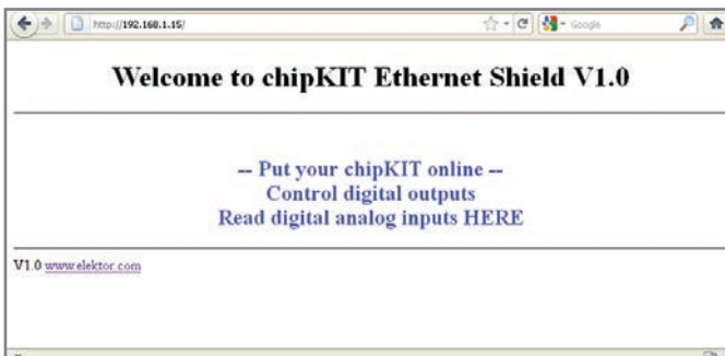
Photo 4 —The result of a successful port: I can now connect to a little web browser running on the chipKIT Max32.
