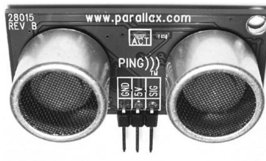
Figure 12-26: The Ping))) ultrasonic distance sensor
