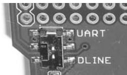
Figure 13-4: GPS shield data switch
