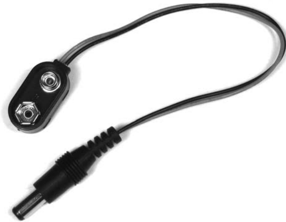
Figure 12-12: Battery cable used to connect the battery to the Arduino
