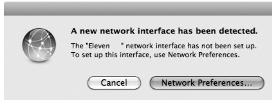
Figure 1-10: A new Arduino board is detected. Your dialog may read Uno instead of Eleven.
