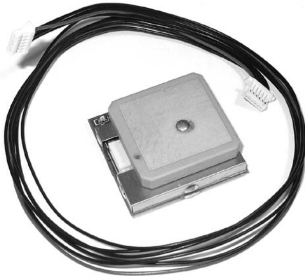
Figure 13-3: A long GPS-receiver-to-shield cable
