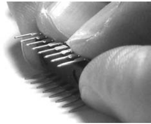
Figure 11-12: Bending the microcontroller pins
