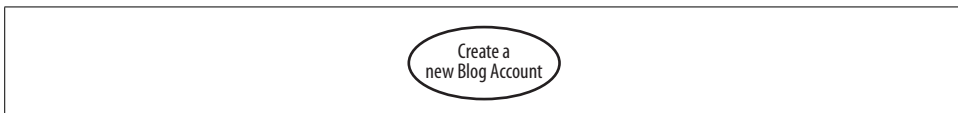
Figure 2-5. A use case in UML is drawn as an oval with a name that describes the interaction that it represents
