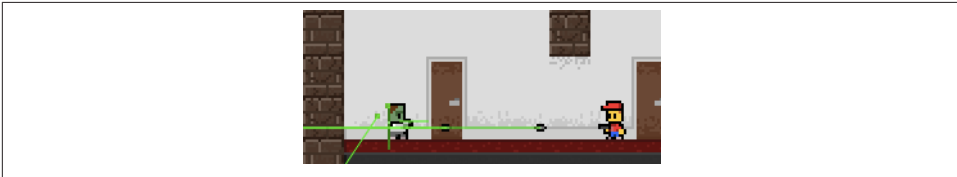
Figure 8-5. Toggle Show Velocities to see green lines that help visualize each entity's velocity as it moves.
