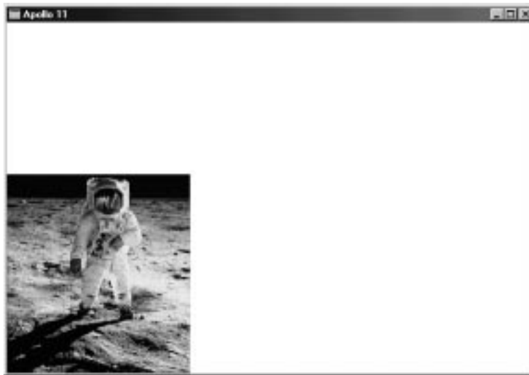
Figure 15-3. A bitmap as it would be displayed under OS/2 with a (0,0) destination.
