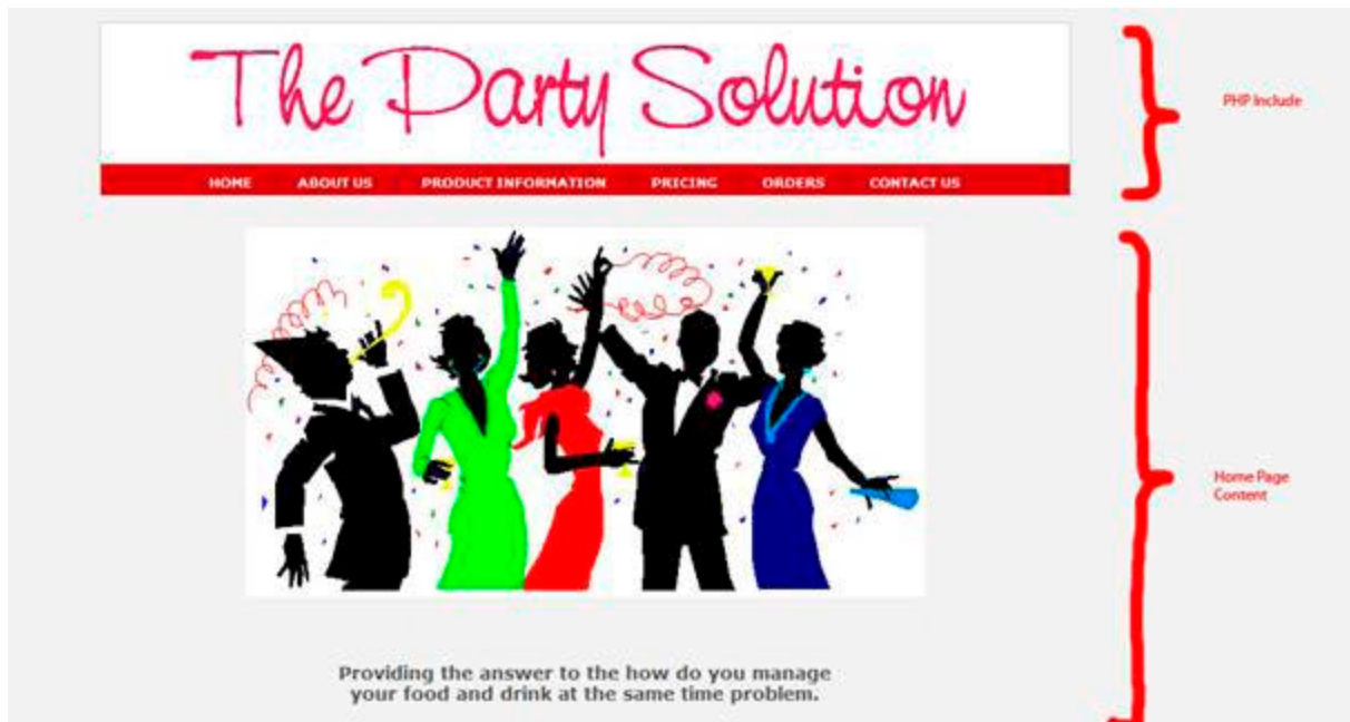
Figure 2. Displaying a common header using a PHP include is easy with Expression Web 2.
