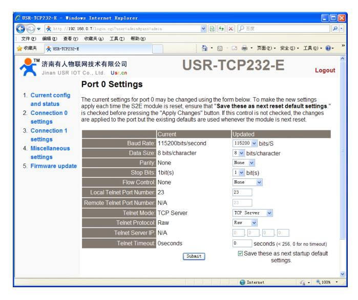
To test briefly in default working mode, on the foundation of the hardware connection, use the matched software USR-TCP232-Test in CD to make transmitting and receiving Test. The left side is serial port, use software default Settings, the right side is the network part, set to TCP client and server to be IP 192.168.0.7, port 23.
