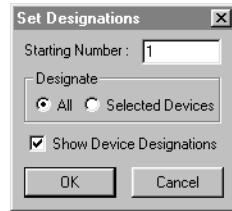
Figure 10.3. Use this dialog box to renumber device designations for all devices or a group of devices.
