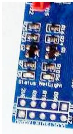
The bright “STATUS” LED will come on, and then the “NETLIGHT” LED will blink once every 800 milliseconds- until the GSM module has found the network, at which point it will blink once every three seconds.
