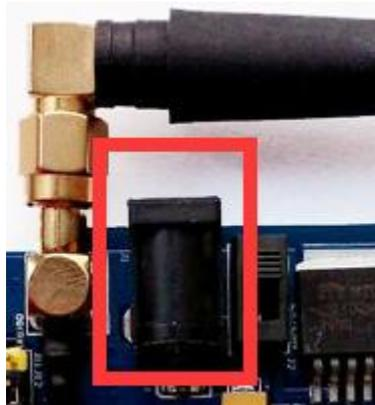
Although the data from Link sprite claims the shield will use no more than 450 mA, the SIMCOM hardware manual (page 22) for the module notes that it can draw up to 2A for short bursts. So get yourself a 5V 2A power supply and connect it via the DC socket, and also ensure the switch next to the socket is set to like the following picture
