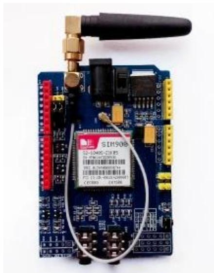
However with a little research and work on your part, the sketches provided *should* also work with any SIM900 module/shield and Arduino – as long as you have the appropriate serial and power settings.
