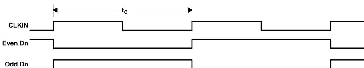
NOTES: A. The worst-case test pattern produces nearly the maximum switching frequency for all of the LVDS outputs.
