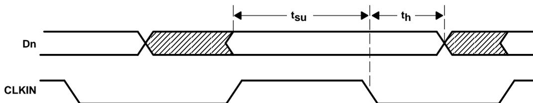
NOTE A: All input timing is defined at 1.4 V on an input signal with a 10%-to-90% rise or fall time of less than 5 ns.
