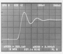
Storage Scope: Risetime is calculated by pushing a single key. Time and voltage differences between cursors are shown on the line above risetime.
