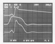
Multiple Storage and Calculation: Volts, current, and power are all shown on the display. Power calculation is a simple keystroke operation.
