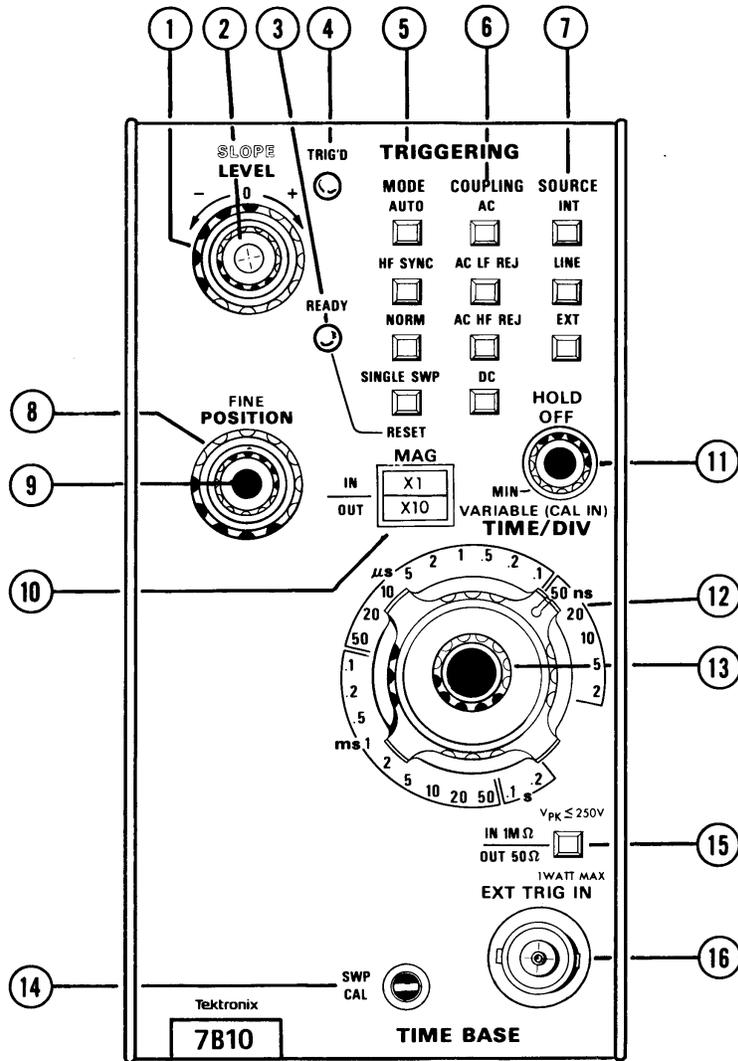
Fig. 2-1. Front-panel controls, connectors, and indicators.
