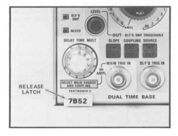
Fig. 2-2. Location of release latch.
