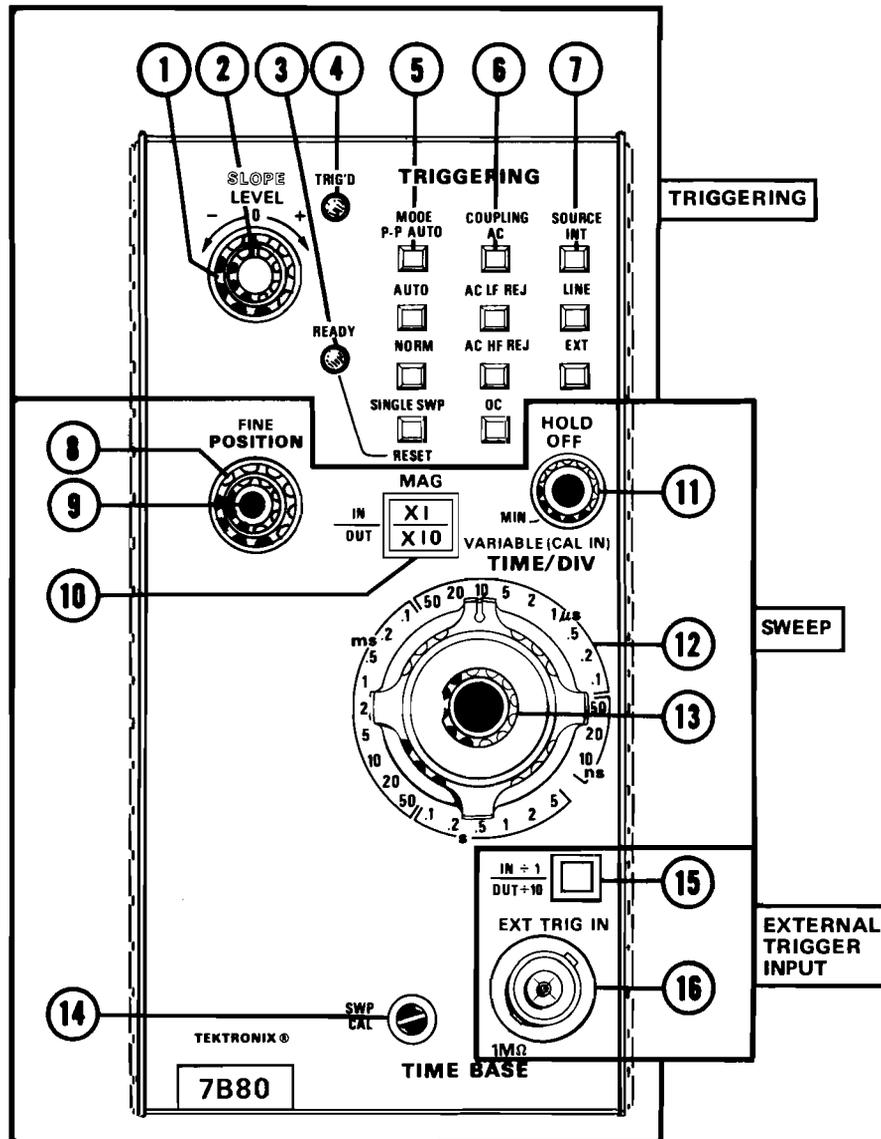
Fig. 1-2. Front-panel controls, connectors, and indicators.
