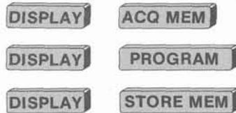
Display commands are executed as soon as the second keystroke in the sequence (the source) is entered. The contents of the source memory are displayed on the Central portion of the display, and a mode change takes place. If the source is Program memory, Programming mode is entered; otherwise, Display mode is entered.
