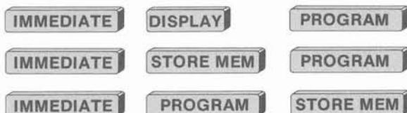
The **IMMEDIATE** key puts the 7D02 into Immediate mode. The second key in each sequence is the destination of the data movement. The third key in each sequence is the source.
