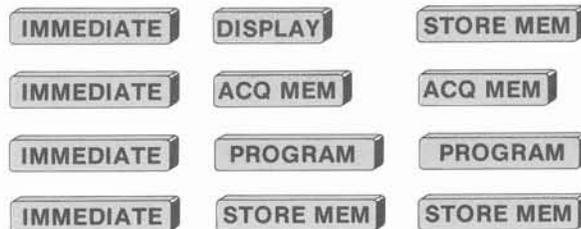
The **IMMEDIATE** key puts the 7D02 into Immediate mode. The second keystroke in each sequence indicates the destination of the data movement. The third keystroke indicates the source.
