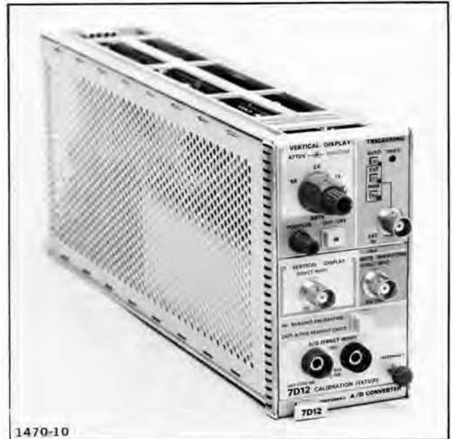
Fig. 4-1. 7D12 Calibration Fixture installed.
