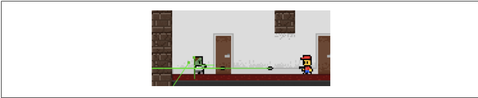
Figure 8-5. Toggle Show Velocities to see green lines that help visualize each entity's velocity as it moves.
