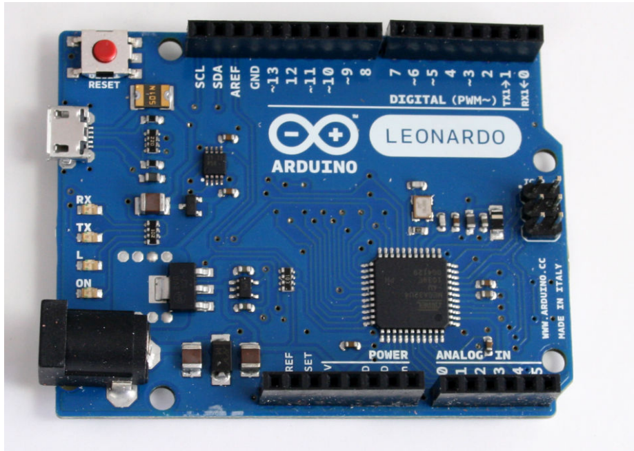
Figure 5-1. Basic board: the Arduino Leonardo
