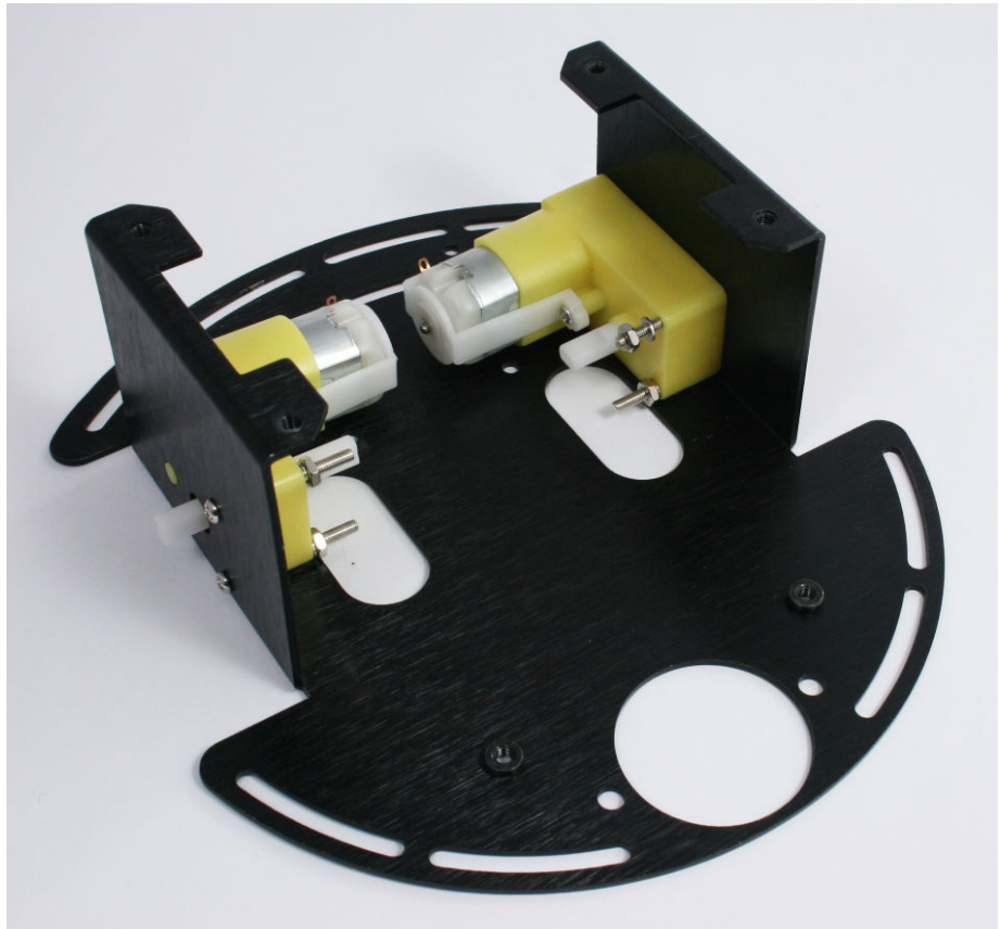
Figure 3-4. Motors mounted on the chassis lower plate
